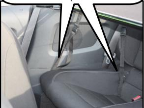
The black snap hook straps will lock into the Child Anchor system. The anchors are located the 4 holes in the rear seats. Then buckle the strap into the wind deflector
