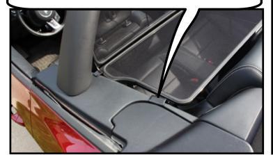
The Wind Deflector is designed to sit under your Lightbar. The wind deflector should not touch your Lightbar. It will be 1/4 inch away.
