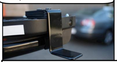
To lower the height of the wind deflector remove 1 or 2 spacers on both sides. this will lower the wind deflector.
