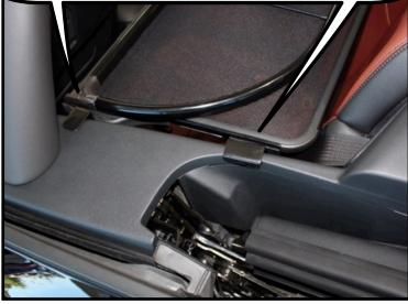
The rear brackets sit on the trim panel in the back seat. The brackets are designed to be used with your boot cover
