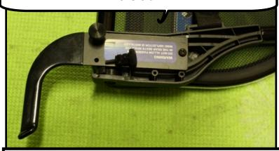
To store the wind deflector in the trunk remove the thumbscrews from the front brackets, then turn the bracket down. Then replace the thumbscrews. Store in the storage bag
