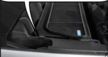
There are 4 straps that hold the wind deflector in place. Two straps use the child anchor system and two attached to the bottom of the trim panel
