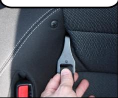
The silver hook straps hook into the cutout on the bottom of the trim panel and then buckle into the bottom of the wind deflector.
