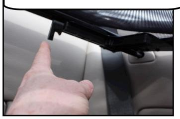
When you are finished please double check that all four handles are turned downwards so the barrel bolts are in the locked position.
