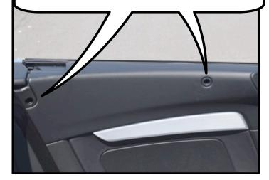
Start by extending both barrel bolts on one end of the wind deflector. Turn the handles so they are facing down, when in the car. This locks the bolts into place. These bolts will slide into the holes on the opposite side of the car from which you are standing.
