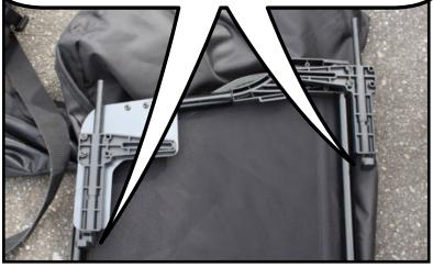
Next, lower the wind deflector into the back seat area and insert the front bolt into the hole into the trim panel and then insert the rear bolt.
