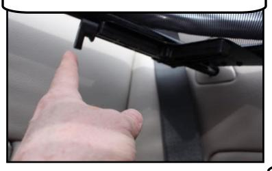
When you are finished please double check to that all four handles are turned downwards so the barrel bolts are in the locked position.
