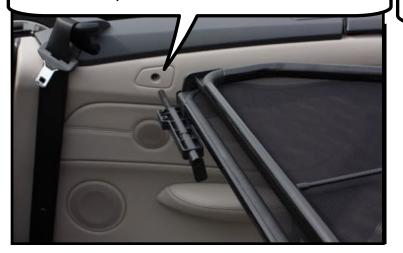
Now lower the wind deflector into the back seat area so the front barrel bolt is in line with the front hole. Slide the bolt forward into the hole and turn the handle down to lock the bolt.
