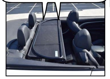
Start by extending the front and rear barrel bolts on one side of the wind deflector. Turn the handles so they will face down, this locks the bolts into place. These bolts will slide into the holes on the opposite side of the car from which you are standing.
