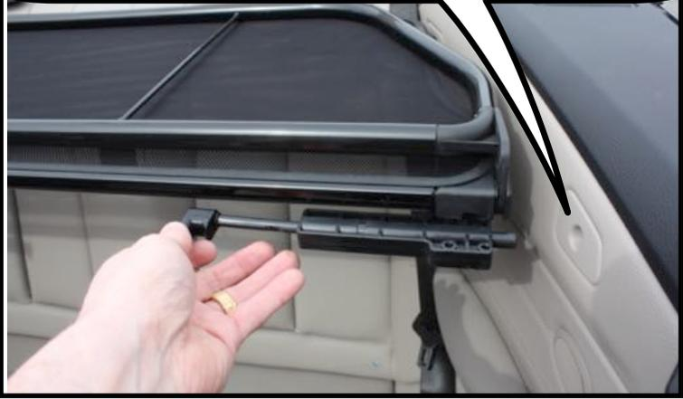
Next, reach back and slide the back bolt into the rear hole and turn the handle down to lock the barrel bolt
