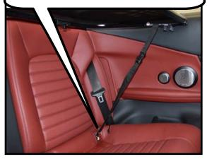
Look for the tabs that has an image of a baby seat and say "ISOFIX". The snap hooks attach to the anchor system behind this Tab
