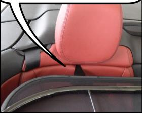
The Front brackets sit on the rear trim panels. The brackets are coated in Plastisol. Which is a soft Vinyl that will not mark the trim panel
