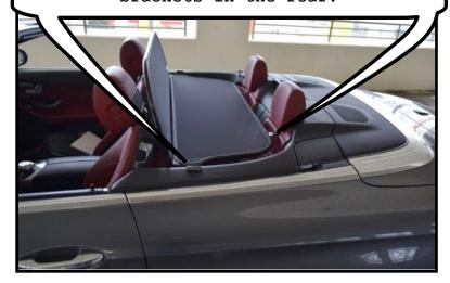
The Rear brackets slide into the slot on in the rear seat. This Slot is located where the rear seat folds down to allow access to the Trunk.
