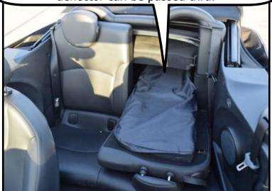
Now lower the wind deflector into the back seat area so the front barrel bolt is in line with the front hole. Slide the bolt forward into the hole and turn the handle down to lock the bolt.
