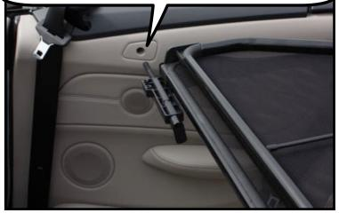
Next, reach back and slide the back bolt into the rear hole and turn the handle down to lock the barrel bolt
