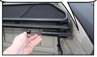
When you are finished please double check that all four handles are turned downwards so the barrel bolts are in the locked position.
