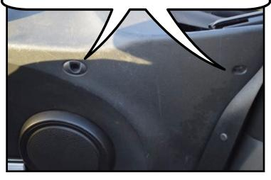
Start by extending the front and rear barrel bolts on one side of the wind deflector. Turn the handles so they will face down, this locks the bolts into place. These bolts will slide into the holes on the opposite side of the car from which you are standing.
