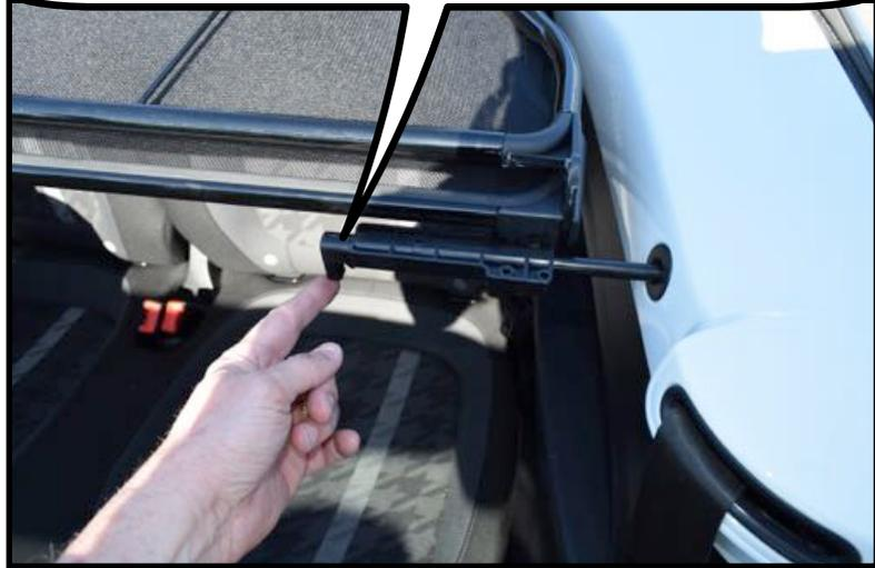
Hold the wind deflector so the barrel bolt is aligned with the hole on the side trim panel.
