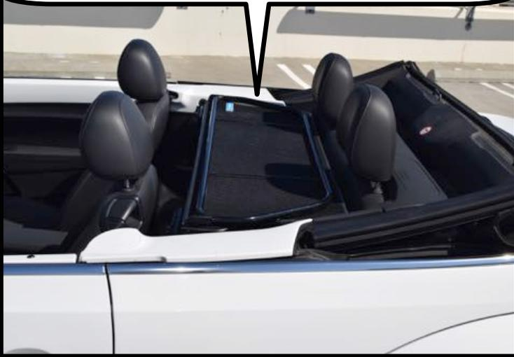
Slide Front bolts into the front holes and then turn the handle down (towards the floor) to lock the handle.
