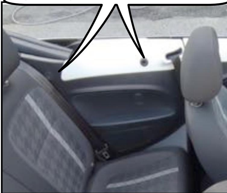
Your wind deflector has four bolts that slide into these holes. Two in the front and two in the rear.
