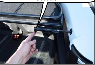
Hold the wind deflector so the barrel bolt is aligned with the hole on the side trim panel.
