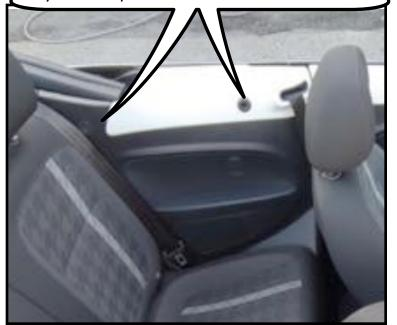
Your wind deflector has four bolts that slide into these holes. Two in the front and two in the rear.
