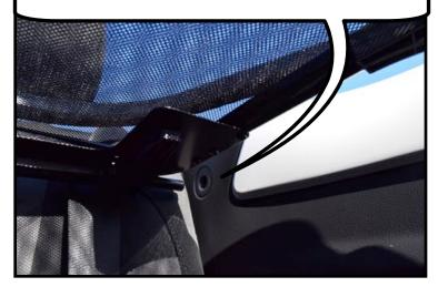
Turn the handle down (towards the floor) to lock the handle.
