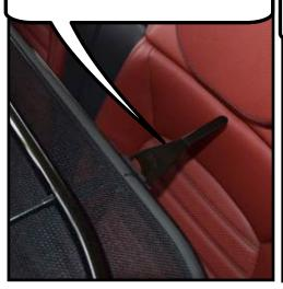
Next lower the wind deflector in the rear seat area. Slide the rear brackets into the slot in the rear seat.
