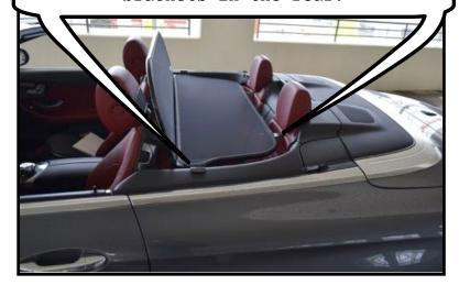
The Rear brackets slide into the slot on in the rear seat. This Slot is located where the rear seat folds down to allow access to the Trunk.
