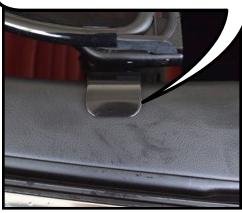
Next attach the two straps that hold the wind deflector in place. These straps attach to the anchor system in the rear seats.
