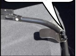
Start by inserting the end of the wind deflector with the rear bracket that has been
