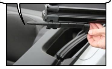
Turn the bolt handle down to lock it in place. Turn the handle towards the front to slide the bolt into and out of the hole.
