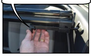
Insert the rear brackets into the rear seat belt slots.
