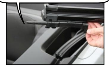
Turn the bolt handle down to lock it in place.
