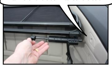
Next, reach back and slide the back bolt into the rear hole and turn the handle down to lock the barrel bolt
