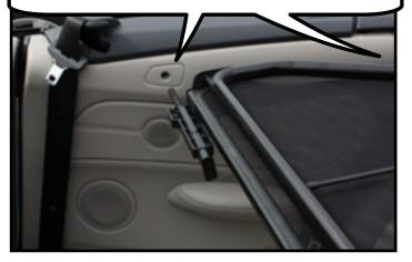
Now, lower your end into the back seat area so the front barrel bolt is in line with the front hole. Slide the bolt forward into the hole and turn the handle down to lock the bolt.
