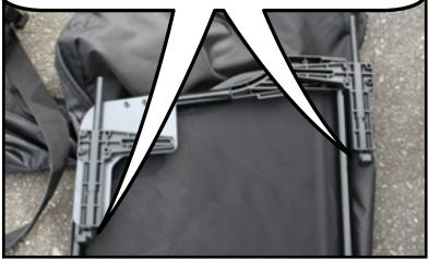
Lower the wind deflector into the back seat area and insert the front bolt into the hole and then insert the rear bolt.
