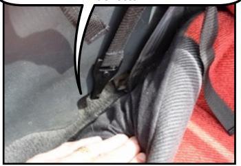
The front strap has a silver hook and attaches to the bottom of the trim panel beside the rear seat. Pull the strap down to tighten the front straps.
