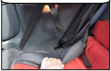
The rear straps are attached to the trim panel beside your rear seat. Pull the bottom panel of the rear seat back and attach the black hook into the cut out of the trim panel. Then pull the strap to secure the wind deflector.
