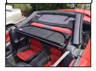
The wind deflector attaches to your convertible and is held in place using 4 brackets and 4 straps
