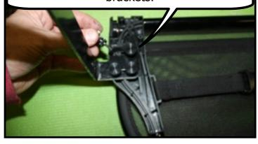
Lay the front brackets flat on the bottom of the wind deflector. The two thumb screws will go into the holes on on the bracket and into the plastic.
