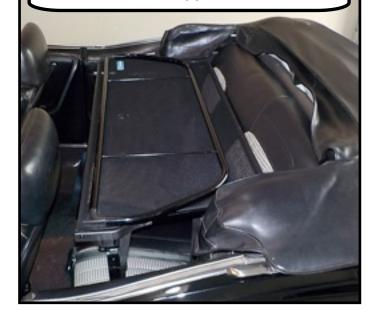
The front brackets are inserted into the ash trays in the back seat. Just slide the ash tray cover open and insert the front bracket into the front part of the ash tray.
