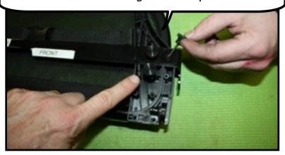
To install the brackets remove the thumb screws and stand the brackets up. Insert the thumb screws into the holes and tighten.
