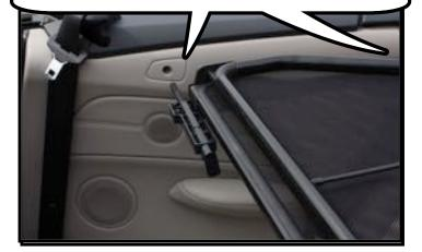
Now lower the wind deflector into the back seat area so the front barrel bolt is in line with the front hole. Slide the bolt forward into the hole and turn the handle down to lock the bolt.
