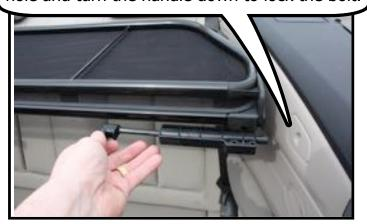
Next reach back and slide the rear bolt into the rear hole and turn the handle down to lock the barrel bolt.
