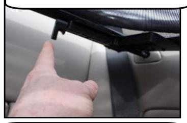
When you are finished please double check to that all four handles are turned downwards so the barrel bolts are in the locked position.
