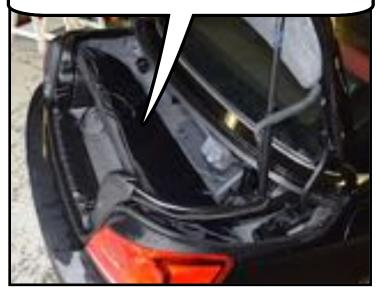
The other option is to use the Passageway between the Trunk and backseat as shown in the photo. But the backseat must be lowered flat so no one can sit the backseat.
