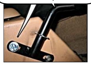
Please note that the tube brackets point toward the back of your Miata. The wind deflector is supported by the shaft bracket and sits behind the
