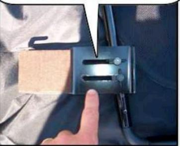
ONCE IN PLACE YOUR WIND DEFLECTOR WILL REST ON THE TRIM PANEL AND LOCK INTO THE SLOTS ON THE SIDE OF THE TRIM PANEL
