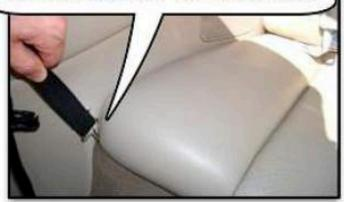
START BY PLACING THE REAR BRACKET ON THE OPPOSITE SIDE, TO WHICH YOU ARE STANDING, INTO THE HOLE ON THE TRIM PANEL
