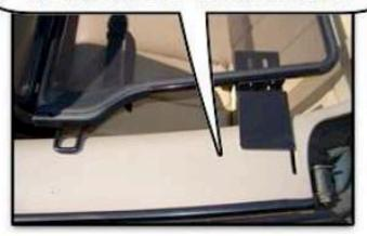
THEN ADJUST THE BRACKET ON YOUR SIDE INTO THE HOLE. LOWER THE WIND DEFLECTOR INTO PLACE
