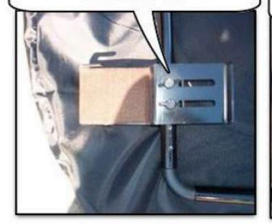
TO INSTALL THE WIND DEFLECTOR START BY LOOSING THE THUMB SCREWS (ONE COMPETE TURN) AND PUSHING BRACKET OUT. TIGHTEN ONE THUMBSCREW LOOSELY. REPEAT ON OTHER SIDE.
