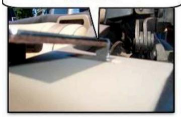
THE LAST STEP IS ATTACH THE TWO FRONT STRAPS. THE STRAPS HOOK TO THE BOTTOM TRIM PANEL JUST IN FRONT OF THE BOTTOM OF THE REAR SEAT
