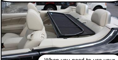
The wind deflector comes with two straps. Attach the two straps with black snap hooks to the Child Anchor system. The Anchors are located at the bottom of your rear seat. Look for to round circles. Slide the hooks in, with the hook facing down, they will lock into place with a snap
