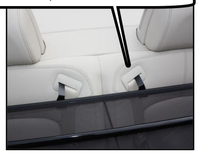
Start by lowering your top and sliding one of the front seats forward. Next aline the rear brackets with the slots for the rear seatbelts. Then slide the brackets into the slots.
