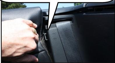
Hold the wind deflector with one hand and lower it so it is even with the rear trim panel
