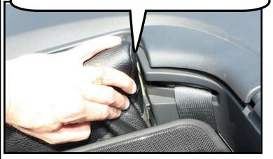
With the handle facing towards the front of the car slide the bolt out and into the hole in the side trim panel.
