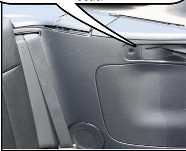
You can find the rear holes by pulling your rear seat to one side to show the holes, they are just below the height of the rear seat belts
