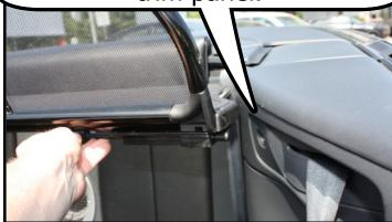
Turn the handle down so it faces the floor, this will lock the bolt into place. Repeat on other side
