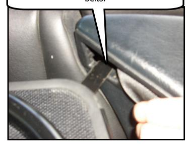
The front brackets of the wind deflector will rest on top of the side trim panel.
