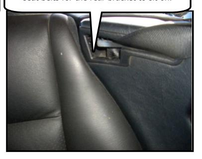
The first step is to stand outside your car beside the back seat and lower the wind deflector into the back seat area. Insert the rear bracket in the space below the seat belt on the opposite side you are standing. Then insert the rear bracket on the side closest to you.
