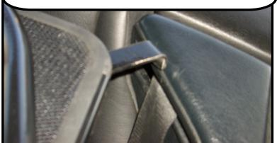
The two brackets should sit flat on the trim panel and not interfere with the rear seat belts.
