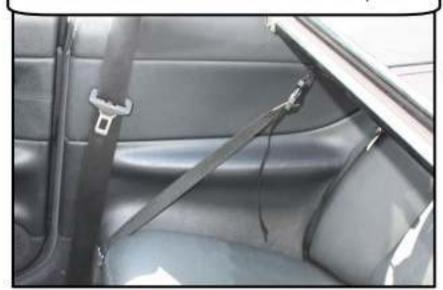
Attach the silver hook to the trim panel beside the bottom on the rear seat. Pull the strap snug, it does not have to be tight. You are now done, flip the top panel of the wind deflector up and enjoy!
