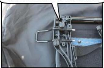
Then flip the brackets around and loosely tighten the thumbscrews. Do NOT tighten the screws so much as to push the bracket into the mesh. Only loosely tighten the thumbscrews.
