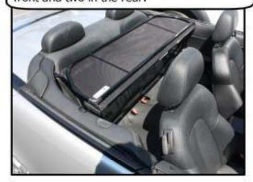
Start by lowering the wind deflector into the rear seat area. The front brackets rest on the side trim panel. The rear brackets will go into the holes where the back seat belts come out of.
