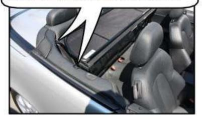
The rear brackets will rest on the seatbelts when you first put the wind deflector into the backseat.
