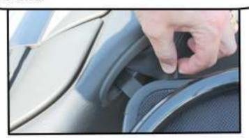
There are two straps on the bottom of the wind deflector that attach to the bottom ofthe trim panel.
