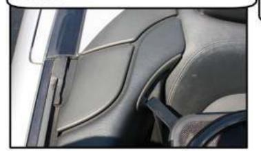
Lift the seatbelt up and allow the rear bracket to hook on to the trim panel. Release the seatbelt and it will cover the rear bracket, repeat on the other side.
