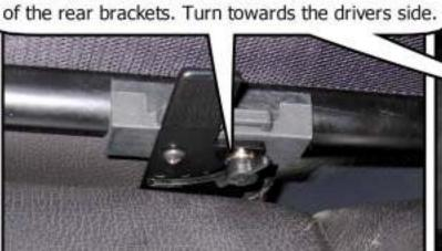
Standing beside the rear seat, lower the wind deflector into the backseat and insert the extended barrel bolt into the hole in the rear trim panel on the opposite side. The rear brackets will rest on the rear seat. Then extend the other barrel bolt into the hole closest to you.
