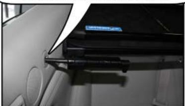
The rear brackets will lock into place around the head rest seat posts. Turning the thumbscrew towards the drivers side will tighten the screws. Turning towards the passenger side will loosen them.
