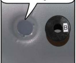
There is a letter "B" on each insert. The letter "B" will point towards the back seat. On the passenger side B will be right side up. On the driver side the "B" will be upside down. But will still be towards the back seat. Tap these in with the palm of your hand or lightly with a hammer. So they are flush to the rear trim panel. You only have to do this once.
