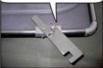
Once both the rear brackets are locked into place, reach under and tighten the thumbscrews on both
