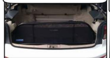
To store the wind deflector, turn handle of the front barrel bolts to the front of the wind deflctor and slide back. Then turn the handle down to lock it. Loosen the thumbscrews (towards passenger side) and close the rear brackets flat.
