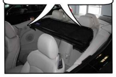
Start by losening the thumbscrews (by one turn) on the rear brackets and turning them so they are at a 45 degree angle like the picture below.
