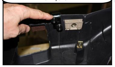
Remove one of the brackets by loosening the large single thumb screw on one end. Then slide the remaining bracket onto the trim panel, close to the middle of the seat belt cover.
