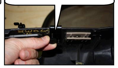
Then attach the large thumb screws on each end to the hole in the wind deflector to the bracket.
