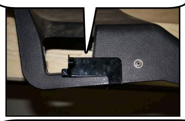
Next tighten the two thumb screws on each side tightly. You might consider using a small pair of pliers. This is a very tight space.
