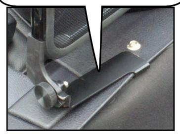
There are two thumb screws that attach the bracket to the trim panel. Start by loosening the thumb screws so there is enough space to slide the brackets onto the trim panel.
