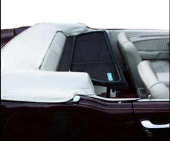
The front brackets are inserted into the ash trays in the back seat. Just slide the ash tray cover open and insert the front bracket into the front part of the ash tray.
