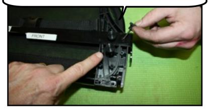
The rear brackets sit on the trim panel in your back seat. Again, the brackets are coated in vinyl so it will not mark your car. Also the brackets are designed to be used with your boot cover if you choose to.
