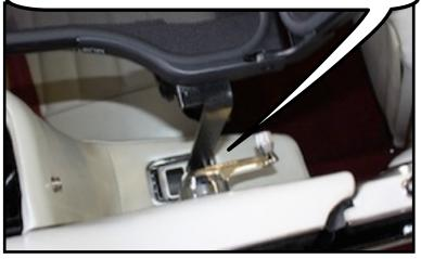
There are 4 straps that hold your wind deflector down. These straps are attached to the bottom of the rear trim panel.
