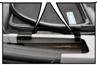
**STEP 2:** Next you need to attach the four straps. The two rear straps with the black snap hooks will clip onto the child seat anchoring system.
