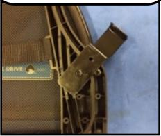
Remove the screw that is not inserted into the bracket. Turn the bracket towards the front of the wind deflector so it is straight.
