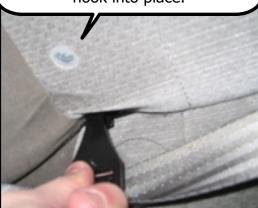
The other two straps will attach to the bottom of the trim panel on each side of the back seats. Once all four of the straps are connected, the wind deflector is installed and you are ready to go.
