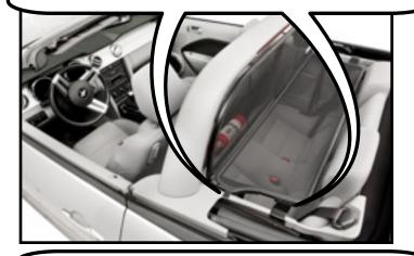
**STEP 1:** Start by lowering the folded wind deflector into the back seat area so the brackets fit onto each side of the trim panel.
