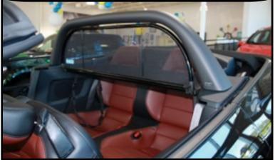
There are 4 straps that hold your wind deflector down. Two use the child anchor system and two attach to the bottom of the trim panel.
