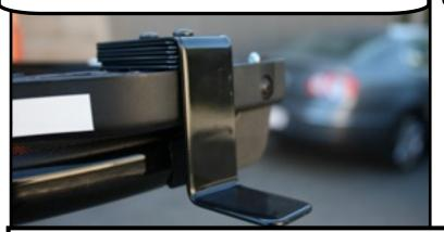
To lower the height of the wind deflector remove 1 or 2 spacers on both sides. this will lower the wind deflector.
