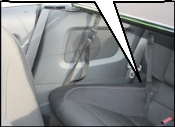
The black snap hook straps slide into the holes in the rear seats. They will lock into the child anchor system. Then buckle to the strap into the wind deflector.
