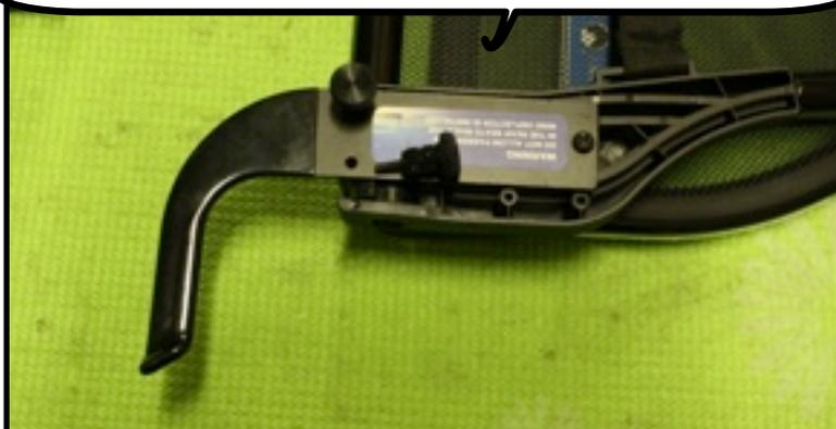
To store the wind deflector in the trunk remove the thumb screws from the front brackets, then turn the bracket down and store in the storage bag.
