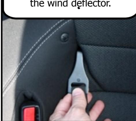
The silver hook straps hook into the cutout on the bottom of the trim panel and then buckle into the bottom of the wind deflector.
