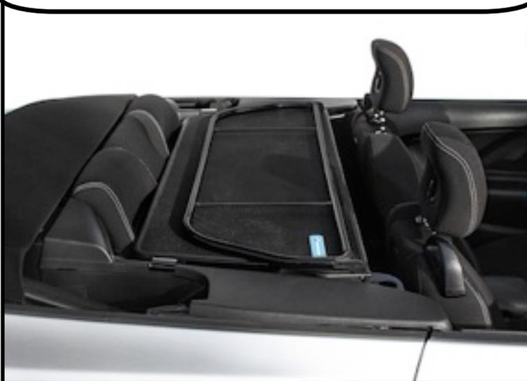
The front brackets slide into the seat belt slots in the rear trim panel. All the brackets are coated in a soft vinyl so it will not mark your Mustang
