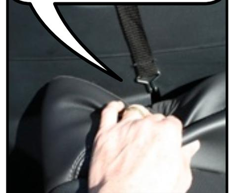
The front brackets have thumb screws to allow the front brackets to turn down for shipping and storing in the trunk.
