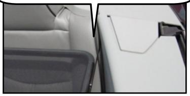
To remove the wind deflector, place one hand on each side of the front panel. Note the back hand is not in the same spot as for installation.
