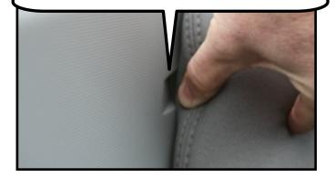
The rear brackets will slide into the holes and the wind deflector will lay flat. The installation is now complete and you can now lift up the top panel.
