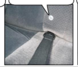
The hooks are inserted with the hook facing down. Then slide the hook in and then pull back to lock it into place.
