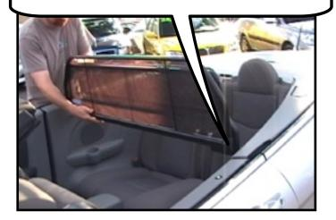
Now, on your side, lower the wind deflector so it lines up with the hole in the trim panel. Slide the locking bolt into the hole and turn the handle downwards to lock it into place.
