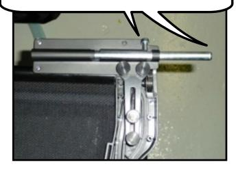
Now, lower the wind deflector into the back seat area. Keeping the wind deflector in an upright position as shown below.
