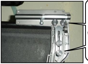
Start by sliding the barrel bolt into the up position. The up position is when all of the thumb screws are below the bolt. Your wind deflector will arrive with the barrel bolts in the up position. Tighten the thumb screws so they are finger tight. The lower position is for storing your wind deflector in your trunk.
