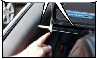
We have made an improvement to your wind deflector. We have added two straps that go from the middle of the wind deflector and attach to child anchor system in the rear seats.
