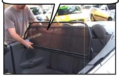
Unfold the bottom panel out towards the rear
