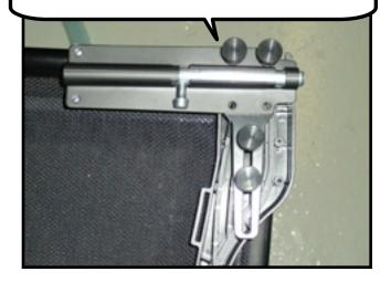
Your wind deflector will fit in the trunk when not is use. Start by folding it up. Then placing the locking bolt side in first.
