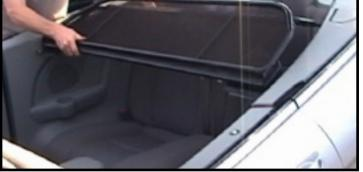
The rear brackets will enter into the holes on each side of the rear trim panel.
