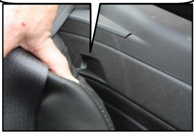
Standing on the drivers side. Flip out the rear bracket on the passenger end. This is what will slide into the slot beside the back seat on the passenger side.
