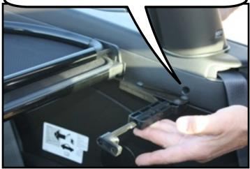
There is also a slot in each side of the rear trim panel beside the back seat. This is where the rear brackets slide into.
