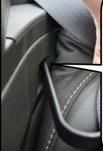
Now lower the wind deflector into the back seat area so the rear bracket goes into the slot beside the rear seat. Then guide the wind deflector so the extended barrel bolt goes into the hole on the passenger side trim panel.
