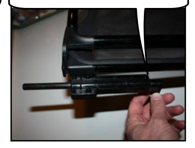
Loosen the thumbscrews on the rear bracket (1 turn counter clockwise (Lefty = Loosey). Turn both of the rear brackets so they face out. Then tighten the thumbscrews by turning them clockwise until they are snug. (Righty = Tighty)
