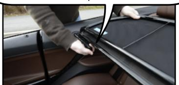
To easily store the wind deflector in the trunk, you will need to lower the barrel bolts. Loosen (do not remove) the thumbscrew at the bottom of the barrel bolt. Remove the top 2 thumbscrews. Slide the bolt down and replace the thumbscrews in the top holes. Reverse the steps to move the bolt to the up position.
