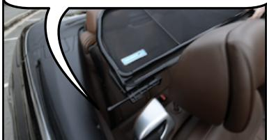
Lower the wind deflector until the barrel bolt on your side aligns with the hole in the trim panel. Slide the bolt into the hole and turn the handle down so it locks the bolt into place.
