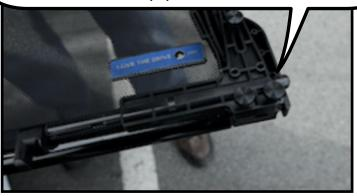
Lower the back of the wind deflector into the holes between the rear seat head rests. To remove the wind deflector just reverse the order of the steps.
