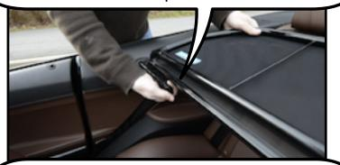
To easily store the wind deflector in the trunk, you will need to lower the barrel bolts. Loosen (do not remove) the thumbscrew at the bottom of the barrel bolt. Remove the top 2 thumbscrews. Slide the bolt down and replace the thumbscrews in the top holes. Reverse the steps to move the bolt to the up position.
