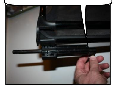
Loosen the thumbscrews on the rear bracket (1 turn counter clockwise (Lefty = Loosey). Turn both of the rear brackets so they face out. Then tighten the thumbscrews by turning them clockwise until they are snug. (Righty = Tighty)
