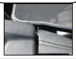
Pull the wire bracket back and forward, then lower it to line up with the space beside the seat belt.
