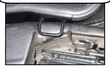
The wire hook, when pulled out, will rest on the trim panel just above the seat belt near the front seats.
