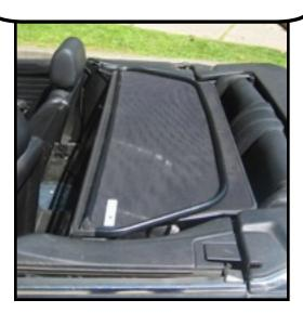
Place the rear bracket behind the dip in the trim panel. Then repeat on the other side.
