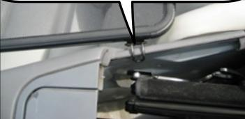
Making sure that both of the black hooks are attached to the trim panel, close the top cover lid to hold the black hooks in place.
