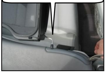
Pull the wire bracket back and lower it so it will line up with the hole in the trim panel.
