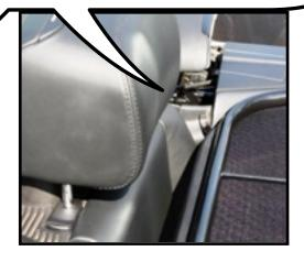
Now on the drivers side, while still holding on to the wind deflector, lower it so the barrel bolt is in line with the hole in the trim panel.
