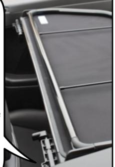
Then slide the plastic barrel bolt into the hole and turn the plastic handle downwards to lock it into position.
