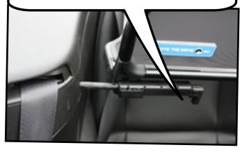
Complete the installation by closing the lid that covers your top completely. The rear brackets will be locked into place by the lid and your wind deflector will sit securely in place.
