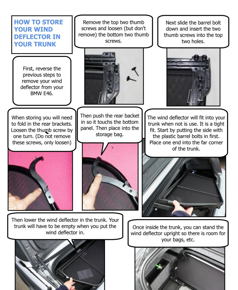
Then lower the wind deflector into the rear seat area so it is flat. The rear brackets will sit on the lip that is below the lid that covers your convertible top. You may need to adjust the rear brackets slightly inward to fit your BMW as each car is a little bit different.
