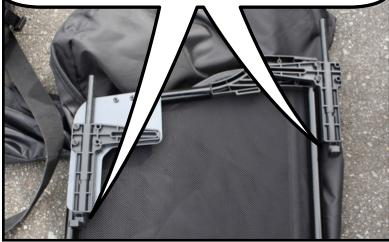
Lower the wind deflector into the backseat area and insert the front bolt into the hole and then the rear bolt.
