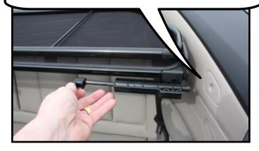
When you are finished please double check to that all four handles are turned downwards so the barrel bolts are in the locked position.
