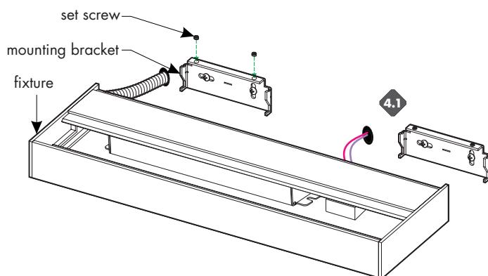
**4.1** Bring in the power wires into the fixture . Align the fixture to the mounting brackets and secure in place using the 2 set screws for each mounting bracket. Use the provided conduit connector if necessary, in accordance with local electrical codes.
