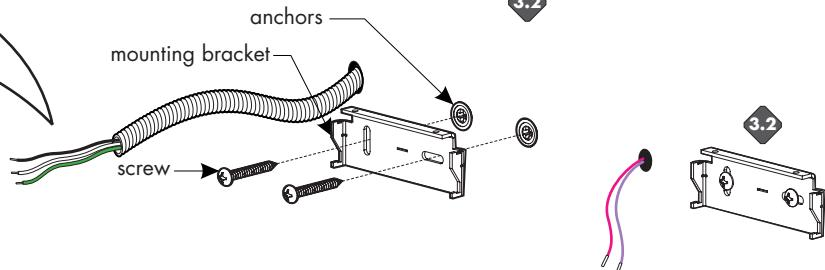
**3.1** Line up the anchors to the marked points. Then tap anchors until the threaded portion. Followed by screwing the remaining with a Phillips screw driver.
