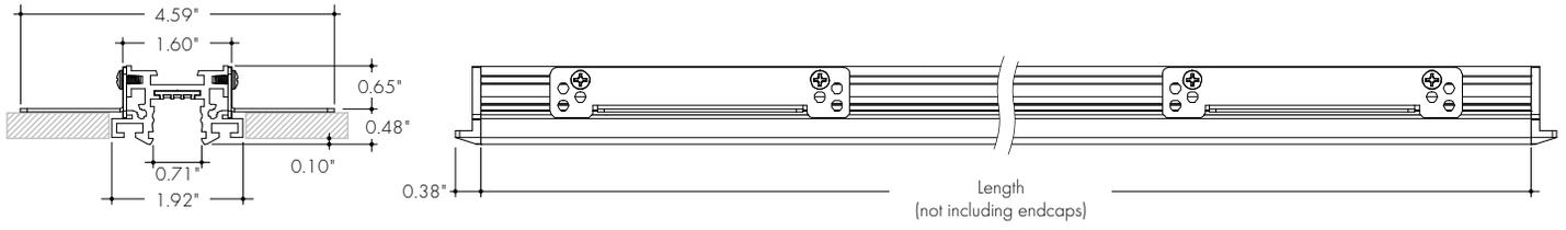
Stenos Track with Directional Module and Louver
