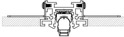
Stenos Track with Ambient Module and Louver
