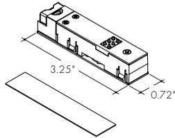
For use with 18AWG field wires with max outer diameter 0.3" (cable and power feed do not ship pre-assembled)
