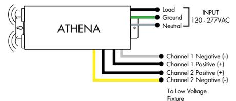
**Track Components (for field configurable systems)**
