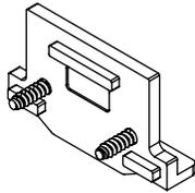
Blank End Cap for ending a Recessed Trimless run
