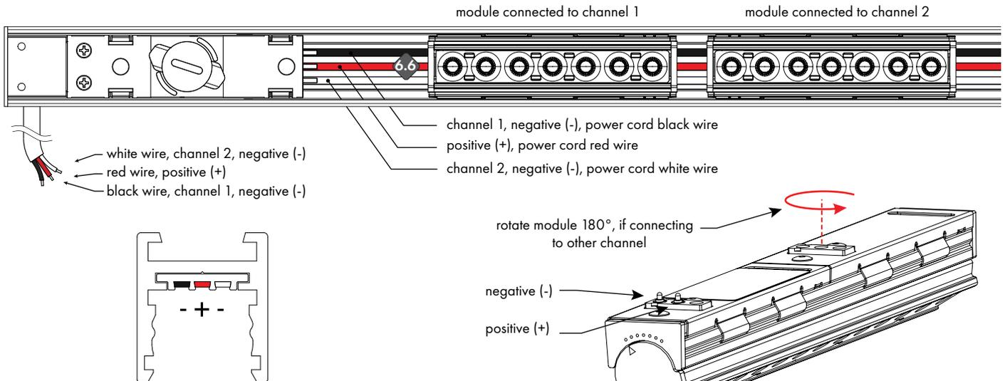
The Power Track contains three copper conductors allowing two channel control .
