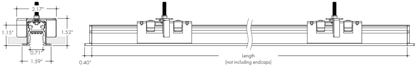
Stenos Track with Directional Module and with louver
