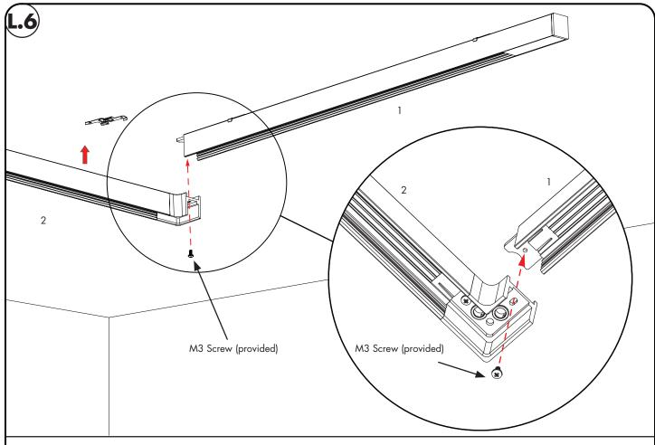
Once track section 1 is attached to the surface, raise track section 2 making sure to line the track up neatly with the mounting brackets.
