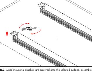
R.3 Once mounting brackets are screwed onto the selected surface, assemble the track section 1 to the mounting brackets. The brackets are rotated in a clockwise direction to lock into the rear of the track.
