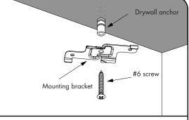
**5.2** For each mounting bracket. Drill a hole into the drywall using 13/64 drillbit and insert drywall anchor. Screw the mounting bracket into the anchor using a #6 screw. If installing to a hollow ceiling or concrete, must use a #6 screw size anchor that is rated for a minimum of 30lbs. For Powerfeed routing, drill a hole into the drywall using 3/8" drillbit.
