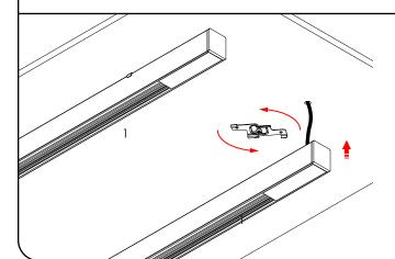
**S.5** Assemble track section 1 to the mounting brackets. The brackets are rotated in a clockwise direction to lock into the rear of the track.
