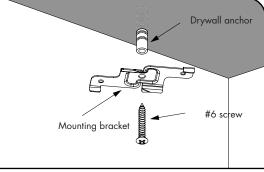
**R.2** For each mounting bracket. Drill a hole into the drywall using 13/64 drillbit and insert drywall anchor. Screw the mounting bracket into the anchor using a #6 screw. If installing to a hollow ceiling or concrete, must use a #6 screw size anchor that is rated for a minimum of 30lbs.
