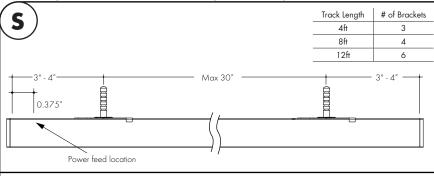
5.1 IMPORTANT! Brackets are to be mounted 3-4" from the end of the track, and spaced apart no greater than 30". Take care to measure and mark where you want to place ceiling brackets before drilling into wall or ceiling
