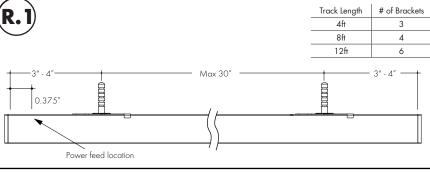
R.1 IMPORTANT! Brackets are to be mounted 3-4" from the end of the track, and spaced apart no greater than 30". Take care to measure and mark where you want to place ceiling brackets before drilling into wall or ceiling
