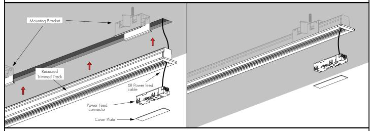
**U.3** Route Power Feed Cable through pre-drilled hole in track and make connection to power supply or junction box (by others). Then insert the track into the mounting brackets to engage the spring clips, securing the track in place.
