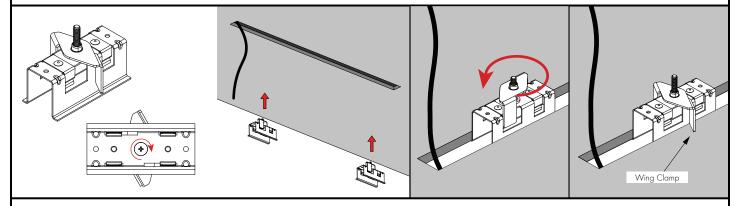
With drywall already installed, create a cutout in the ceiling 1-1/16" wide by (track length + 3/8") length. Take great care when cutting open the channel as you will only have 0.18" lip on the mounting bracket. Refer to approved Custom Layout Drawing by Luminii for precise ceiling cutout dimensions. Insert the mounting brackets into the ceiling cutout. Turn screw to rotate wing clamp and tighten until mounting bracket is secured to the ceiling.
