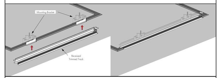
Insert track section 1 into the mounting brackets to engage the spring clips, securing the track in place.
