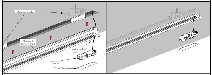
**S.3** Route Power Feed Cable through pre-drilled hole in track and make connection to power supply or junction box (by others). Then insert the track into the mounting brackets to engage the spring clips, securing the track in place.
