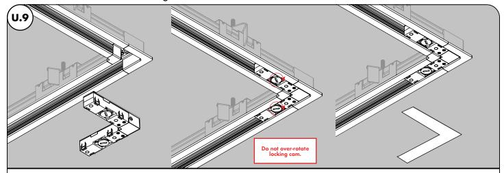
Perform a continuity check between the track conductors and the power cable to ensure that the power feed/joiner is sitting properly in the track.
