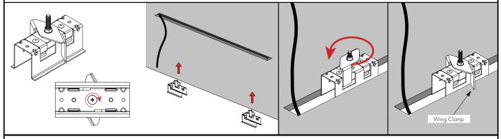
**L.2** With drywall already installed, create a cutout in the ceiling 1-1/16" wide by (track length + 3/8") length. Take great care when cutting open the channel as you will only have 0.18" lip on the mounting bracket. Refer to approved Custom Layout Drawing by Luminii for precise ceiling cutout dimensions. Insert the mounting brackets into the ceiling cutout. Turn screw to rotate wing clamp and tighten until mounting bracket is secured to the ceiling.
