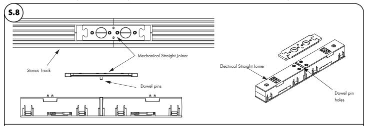
5.8 Align Electrical Straight Joiner dowel pin holes with dowel pins of Mechanical Straight Joiner
