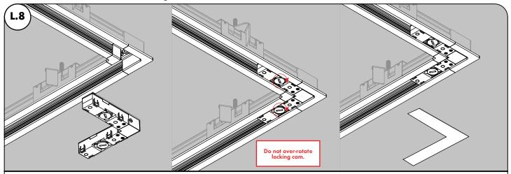
Perform a continuity check between the track conductors and the power cable to ensure that the power feed/joiner is sitting properly in the track.
