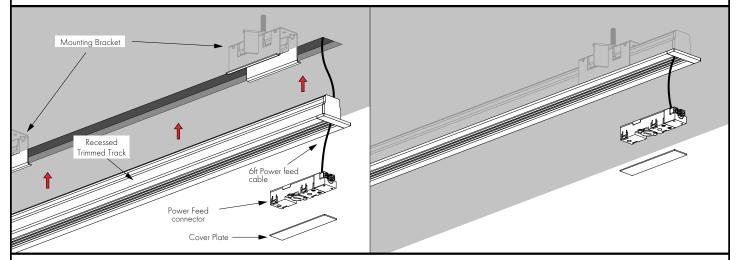
**L.3** Route Power Feed Cable through pre-drilled hole in track and make connection to power supply or junction box (by others). Then insert the track into the mounting brackets to engage the spring clips, securing the track in place.
