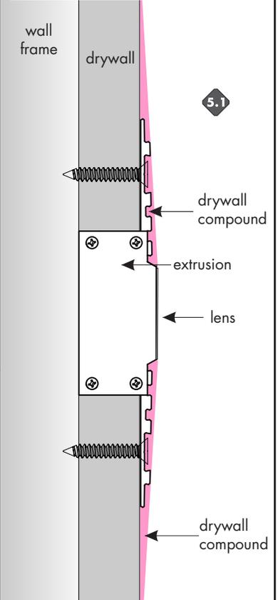
**5.1** Place a coat of durabond on each side of the extrusion (reference diagram to the right) for a strong bond. Followed by a light sand to blend to the drywall. If necessary finish any imperfections with a light compound. Then paint to complete installation.
