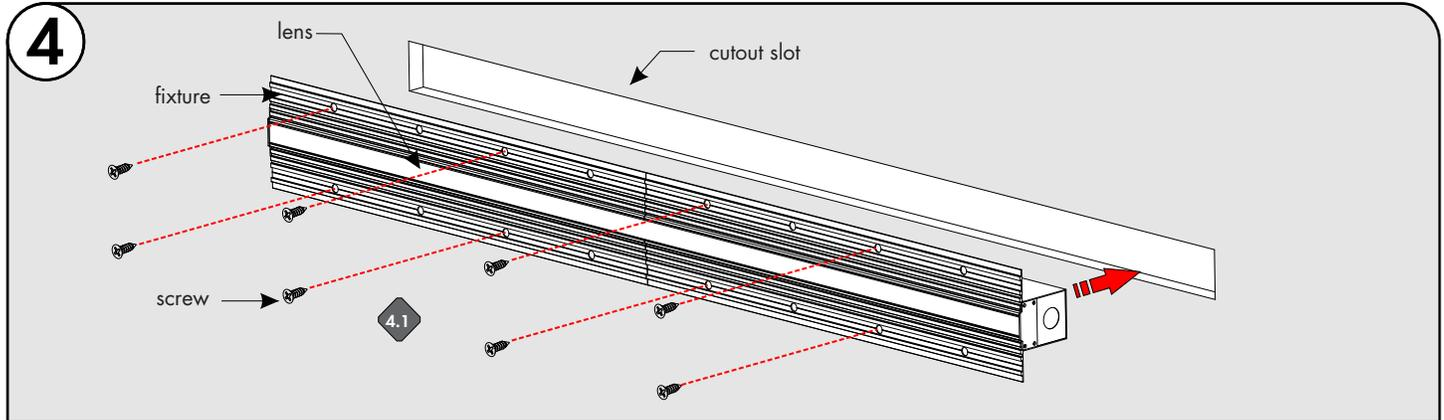
**4.1** Install Slot fixture into ceiling/wall cutout. Be sure to align the end of the Slot fixture with the end of the cutout. Insert the lens into fixture slot. Then Mount into drywall with #8 Drywall Screws.
