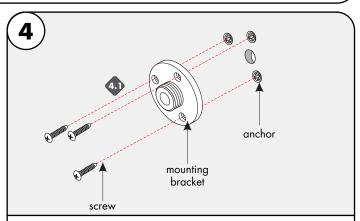
Secure each mounting bracket onto the anchors using the appropriate hardware.
