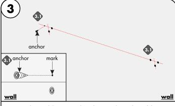
Align and then tap each anchor onto the marks until the threaded section. Followed by tightening the anchors with a Phillips screw driver. (Anchors not provided)
