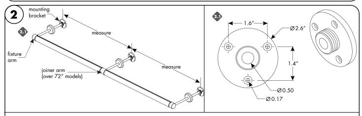
2.1 Measure the distance from one mounting bracket to the next. Then mark these location to the wall. Use the reference detail of mounting bracket above, for any additional information.
