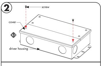
2.1 Remove the two Phillips screws from the top of the driver housing and pull the cover off to expose the driver wires.
