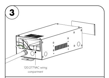
3.1 Connect the white (neutral) and black (hot) power supply wires to the white and black power wires ( 120 - 277 VAC). Followed by connecting the ground wires in accordance with local electrical codes.
