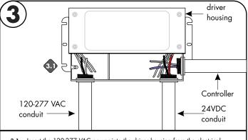
3.1 Insert the 120-277 VAC power into the driver housing from the electrical panel. Followed by bringing the 24V DC low voltage wires from the LEDs into the driver housing. In addition bring the controller wire if applicable. Refer to diagram on page 2 to make all the proper wiring connections.
