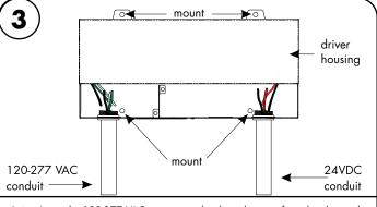
3.1 Insert the 120-277 VAC power into the driver housing from the electrical panel. Followed by bringing the 24V DC low voltage wires from the LEDs into the driver housing. In addition, connect the Triac / Phase dimmer at input if applicable. Refer to diagram on page 2 to make all the proper wiring connections.
