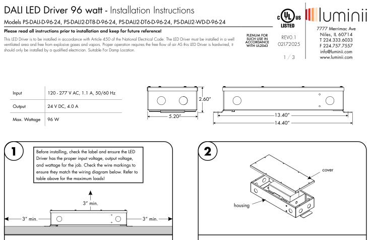
**1.1** LED Driver can be mounted vertically or horizontally. With a minimum of 3" clearance around LED Driver to provide proper air circulation.
