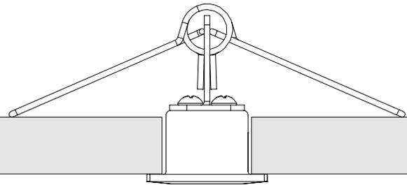
**4.2** For soft surface mounting bracket option: Bend the adjustable springs to a straight position, followed by pushing the fixture completely inside the cutout slot. Then release the springs to secure.
