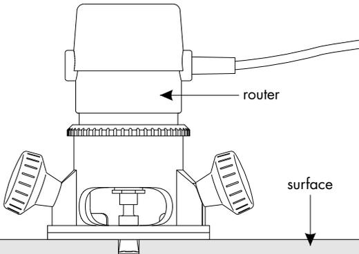
**2.1** Route slots onto the surface with the proper width and depth to accommodate aluminum extrusion. Use drawing above as reference.
