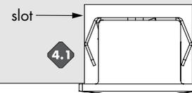
**4.1** For hard surface mounting bracket option: Align the mounting brackets to the cutout slot, then carefully push the fixture completely inside to the slot to secure.
