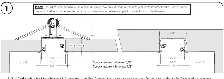
On the left is the Myka Recessed Asymmetric with the Gypsum Mounting spring brackets. On the right is the Myka Recessed Asymmetric with the Hard Surface Mounting brackets.
