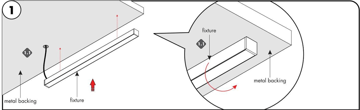
**Note:** : Prior to installation all 24VDC wires must be present near fixture. Refer to the power supply installation instruction for additional information.
